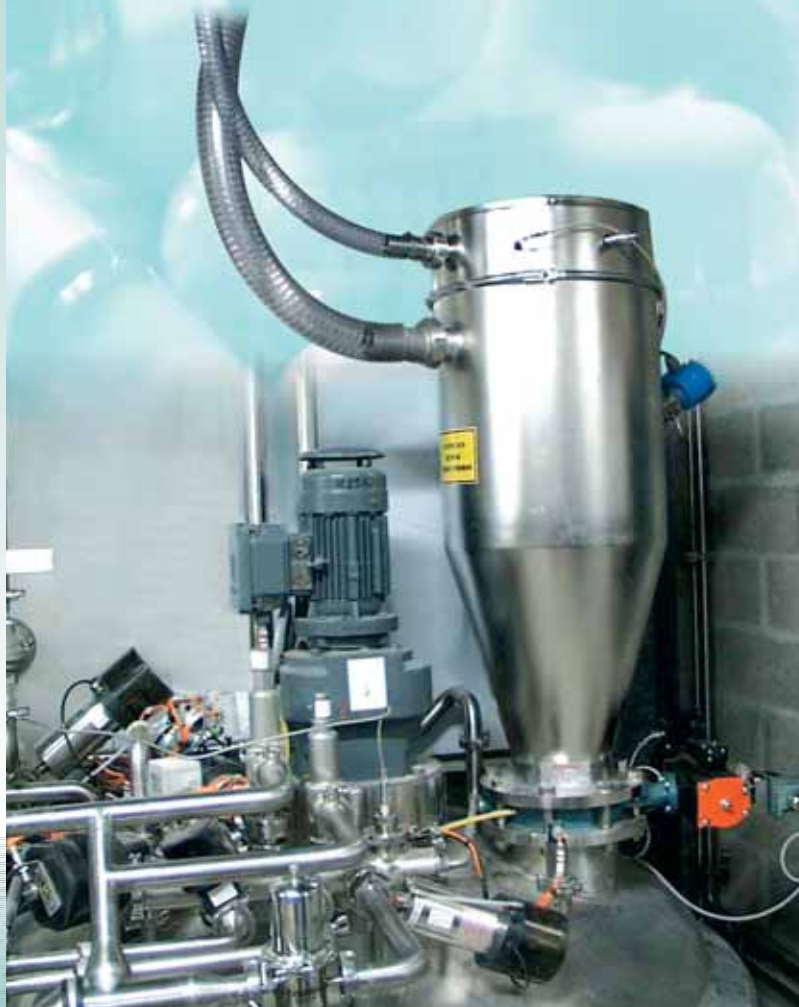
Easy dismantling by clamp collars
